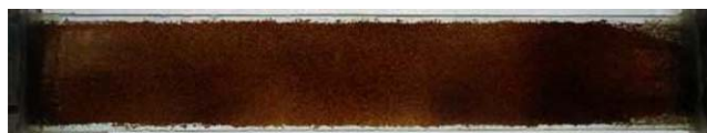
Figure 7. Appearance of ground glass model after oil saturation. [Color figure can be viewed in the online issue, which is available at wileyonlinelibrary.com .]
