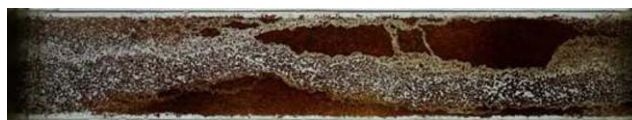
Figure 8. Sweep area change of ground glass model after water flooding ends. [Color figure can be viewed in the online issue, which is available at wileyonlinelibrary.com .]
