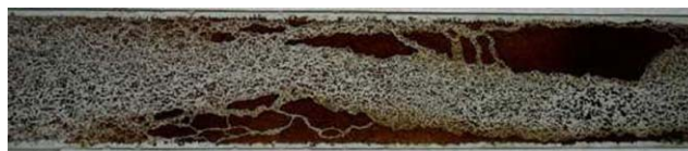
Figure 9. Sweep area changes of ground glass model during injection of 600 mg/L CPAM \mu\text{m} microspheres after swollen for 5 days at 50 °C. [Color figure can be viewed in the online issue, which is available at wileyonlinelibrary.com .]
